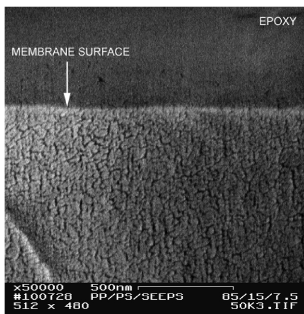
Fig. 2. Scanning electron micrograph of the cross-section of PP/PS/SEEPS blends, PP/PS/SEEPS-85/15/7.5-2 (from Ref. [2]).
